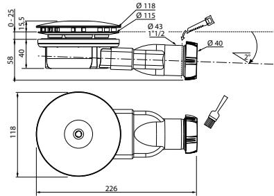
Shower tray siphon, ultra compact 40 mm, with odor-proof membrane antimiros + hair filter, water flow rate of 24 L/min, outlet Ø 40 mm, chrome ABS grate, integrated slope of 2°
