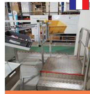
Assembly Setting up a secure platform on the NEO Machine to ease part supplies, thus reduce Musculoskeletal Disorder
