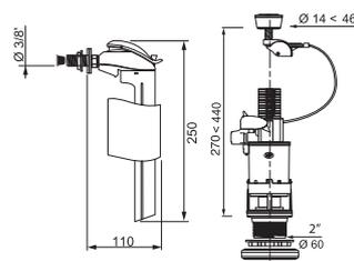
Mécanisme à câble MW<sup>2</sup> + robinet JOLLYFILL FL150
