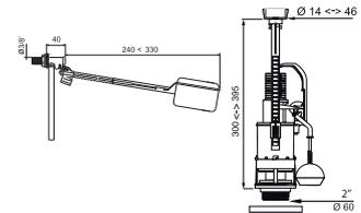
Mécanisme à câble MW<sup>2</sup> + robinet F90
