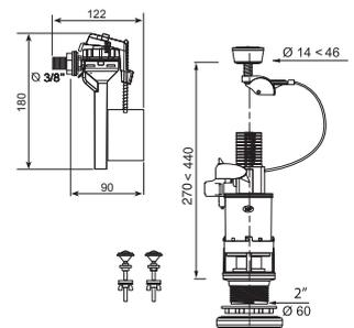
Mécanisme à câble MW<sup>2</sup> économie d'eau + robinet KOMPACT 3/8" semi-laiton
